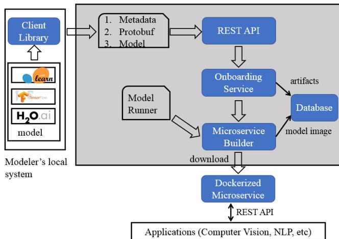
Fig. 3. The Acumos Onboarding System Architecture
